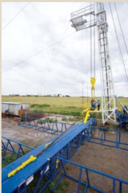
Hydra-Walk automates the pipe-handling process using a mechanical arm to lift pipe lengths from the catwalk and present them to the rig floor.
