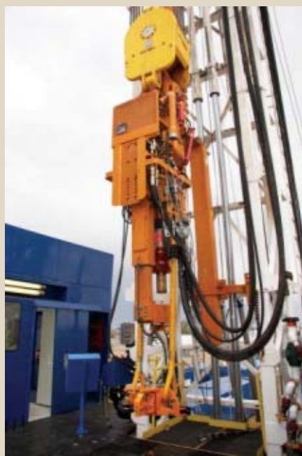
This top drive is symbolic of renewed horizontal drilling and re-entry efforts by Key Energy Services to help customers reach untapped pockets of oil and gas.
